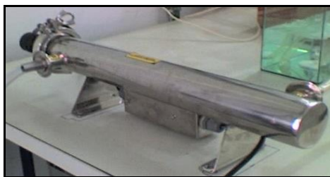
Figure 1: Tubular Reactor Used for Photochemical Treatment
